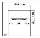
The panel must be fitted with a handle, as the dishwasher handle will be hidden by the panel.
